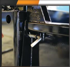
Optional dropside with double spring pins. Side drops well below deck level for easy clean out.
