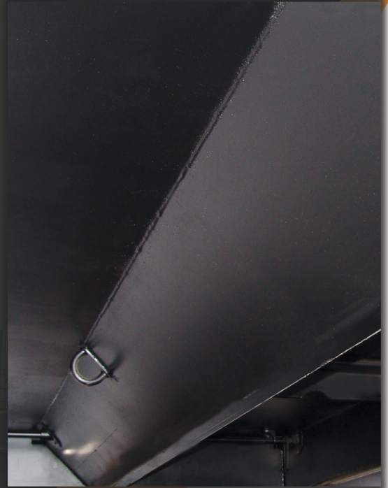
Pictured is the crossmemberless understructure of the 530 and 533 body using 3/16" X 100K formed 11" trapezoidal longbeams
