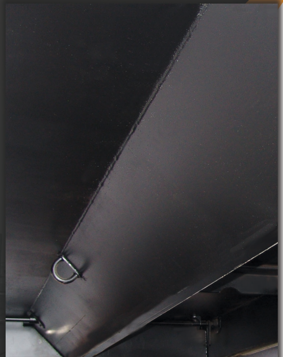
Pictured is the crossmemberless understructure of the 430 and 433 body using 3/16" X 100K formed 10" trapezoidal longbeams
