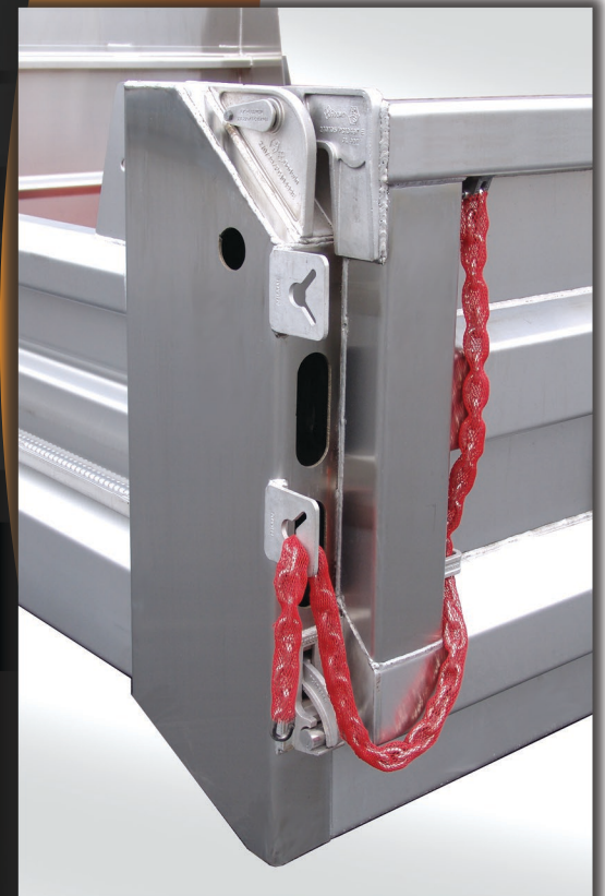
These bodies feature full depth rear corner posts, double chain adjusters, and 7 gauge construction. The 433U uses all stainless hardware
