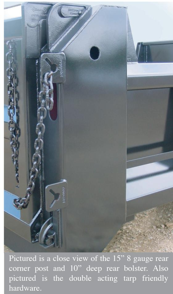
Pictured is a close view of the 15" 8 gauge rear corner post and 10" deep rear bolster. Also pictured is the double acting tarp friendly hardware.
