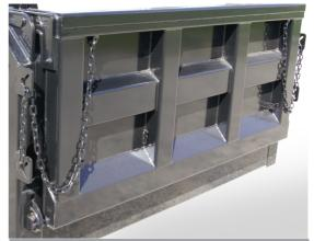
Pictured is the 8 gauge high tensile steel 6 panel tailgate with chains and chain adjustors.
