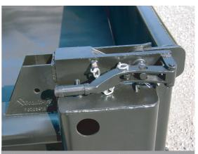
Pictured is a close view of the upper quick release hardware. This hardware makes it easy to quickly remove and reinstall the tailgate.
